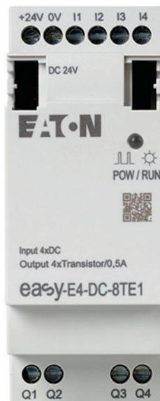
**EXTENSION E/S, 24 V DC, 4 ENTRÉES TOR, 4 SORTIES TRANSISTOR**
